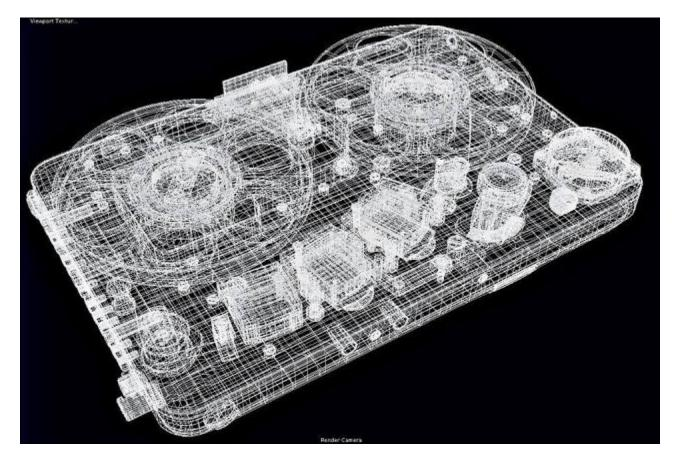
In 1958 the NAGRA III sees the light of day. It is a solid-state machine employing an electric motor with closed loop servo speed control. It is a fully transistorized machine with all the modules enclosed in metal cases. It is powered by conventional "D" type batteries. Moreover, it is equipped with a true peak meter called a "Modulometer". Orders come flooding in and 240 NAGRA III
